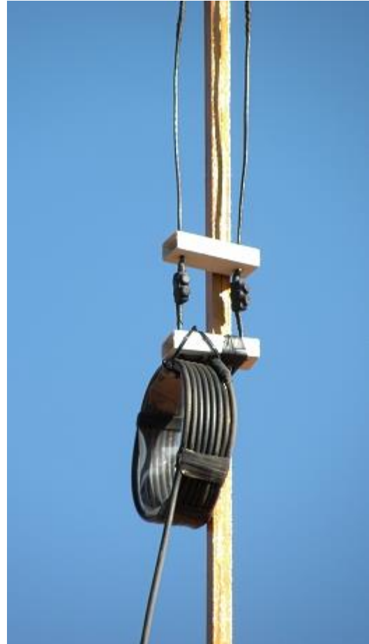
11 m Band "Zepp" (EDZ) antenna: Balun Corrente
